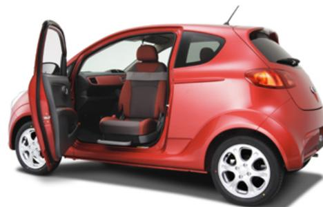
Subaru R1 TransCare Wing Seat (Prototype)
